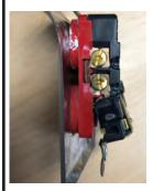
• Recently, the electrical plug pictured here was damaged when a bed was moved while the electrical cord was still plugged in.
